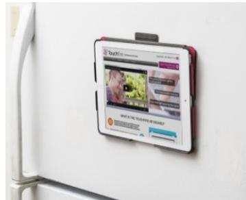
Touchfire's built-in magnetic mount allows the iPad to stick to any ferrous metal, such as a refrigerator or a metal-backed whiteboard.
